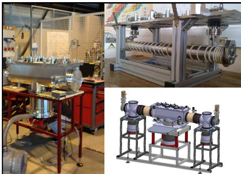
Figure 6: Left: main chamber of the GPIB with the central pump being tested at the CENBG. Upper right: main body of the GPIB showing the DC electrodes. Lower right: illustration of the full GPIB mounted on its HV platform with the lateral pumps.
