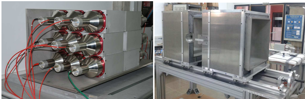
Figure 12: Left: assembly of 18 NaI(Tl) detector modules. Right: radiation shielding plus support table.
