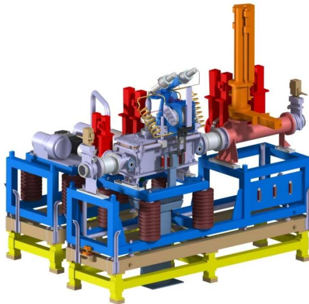
Figure 2: Design of the cooler taking into account all requirements for its use in a high-radiation environment (yellow zone).
