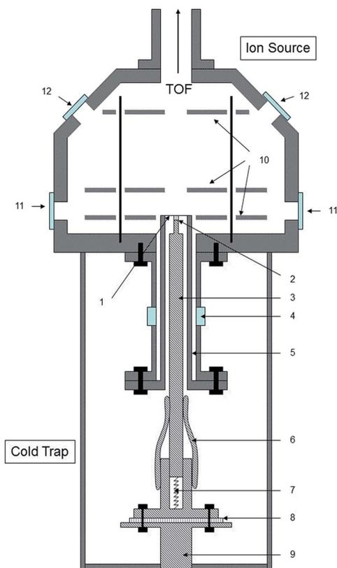
Fig. 3 Schematic of the cold trap and ion source: 1 – thin stainless-steel end, 2 – indium, 3 – copper insert, 4 – insulating ceramic, 5 – re-entrant tube, 6 – copper heat wick, 7 – spring, 8 – insulating sapphire, 9 – cold head, 10 – electrostatic plates, 11 – UV view ports, 12 – IR view ports.
