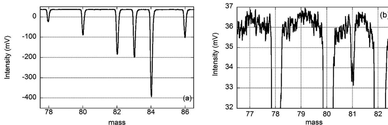
Fig. 7 (a) Kr spectra of the Boguslavka meteorite obtained with 20% of the released gas. Gain is divided by 2 compared to (b) to ensure a signal less than 500 mV and linearity (b) zoom on the  $^{81}\text{Kr}$  signal from 80% of the released gas. The  $^{81}\text{Kr}$  signal corresponds to  $\sim 6700$  atoms and the noise amplitude is  $\sim 750$  atoms.
