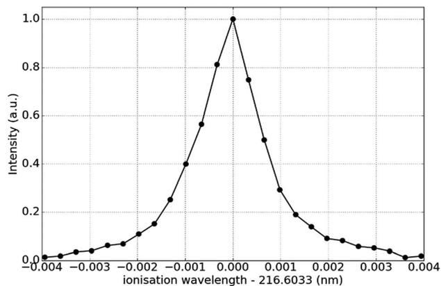
Fig. 6 Influence of the ionization laser wavelength on the  $^{84}\text{Kr}^+$  signal.
