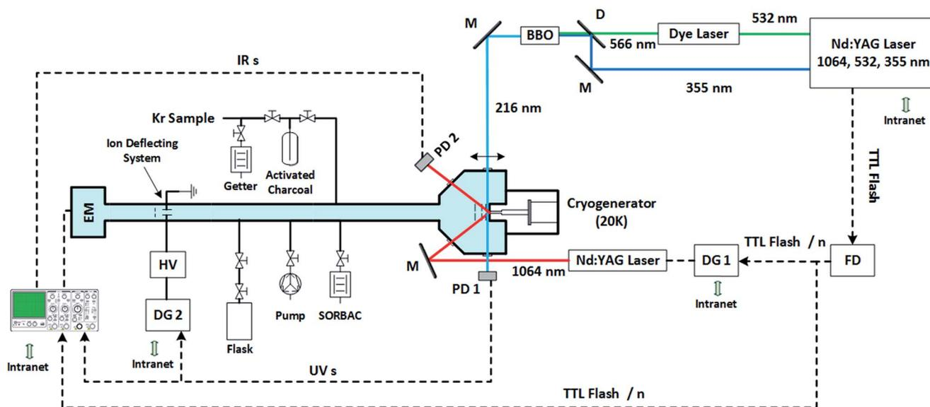
Fig. 1 Experimental set-up. M: mirror, D: dichroic, FD: frequency divider, DG: delay generator, PD: photodiode, EM: electron multiplier. HV: rapid high voltage. Flask: air standard calibration. IRs, UVs: infrared, UV photodiode signals. SORBAC®: gas purification.
