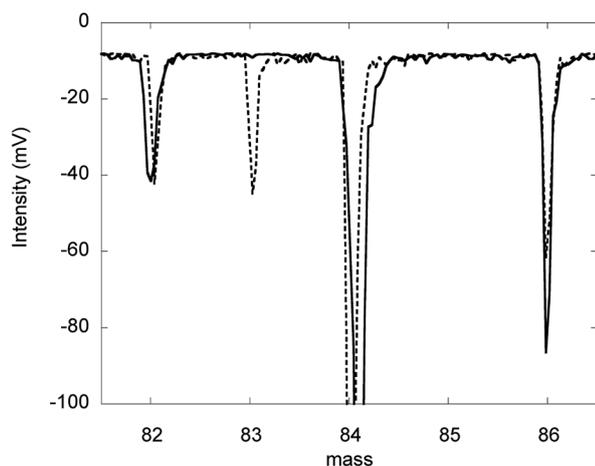
Fig. 4 Spectra of an atmospheric Kr sample obtained without deflecting voltage (dashed line) and with deflecting voltage (solid line) applied to  $^{83}\text{Kr}$ .
