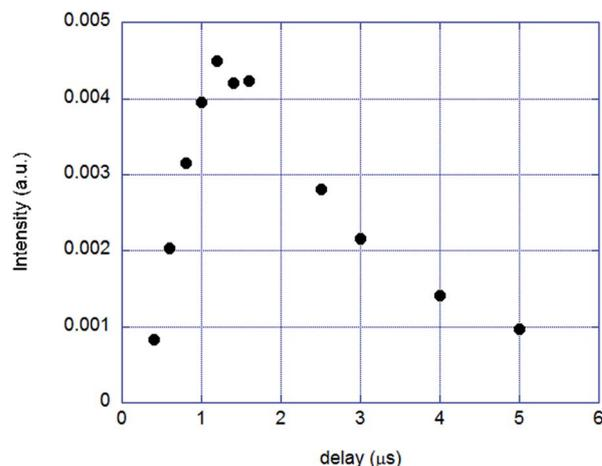
Fig. 5 Kr signal intensity against the inter-laser delay. The maximum ionization is obtained for a delay of 1.5  $\mu\text{s}$ .
