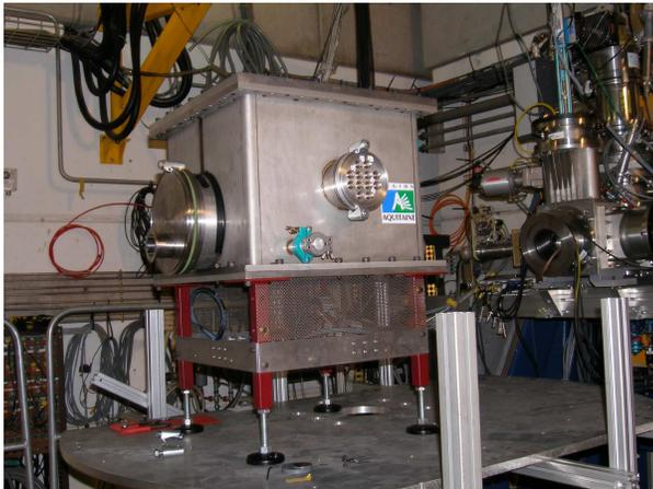
Fig. 7. The TPC installed at the exit of the LISE3 beam line of GANIL.
