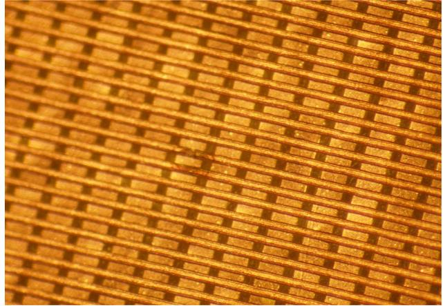
Fig. 4. Photo of the 2D detector composed of a copper-coated kapton foil of thickness  $50\mu\text{m}$  on which the strips have been etched on the upper and lower side. The top strips have a pitch of  $100\mu\text{m}$  and a width of  $50\mu\text{m}$  and are connected on both ends two-by-two. The lower-side strips have a pitch of  $200\mu\text{m}$  and a width of  $150\mu\text{m}$ . The copper thickness on both sides is  $5\mu\text{m}$ .
