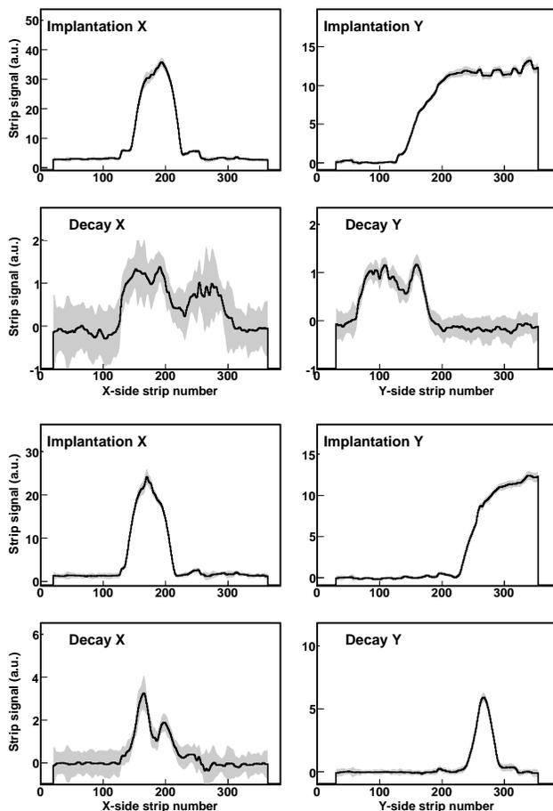
Fig. 8. Two implantation and correlated decay events are shown for  $^{45}\text{Fe}$ . The figures show each time the implantation signal on the X and Y strips and the decay signal on the same strips just below. The decay events start where the implantation trajectory ends. In all cases, the tracks of the two protons can be clearly seen.
