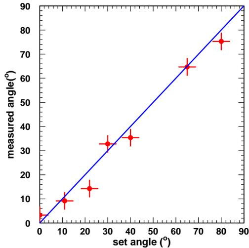
Fig. 5. Drift time calibration as performed with  $\alpha$  particles entering the detection volume under fixed angles. With the known drift time which depends on the nature of the gas, its pressure and the drift voltage, the time delay between the strips can be converted into a drift distance and thus into an angle of a trajectory with respect to the detection plane. The angle resolution obtained is 7-8°.
