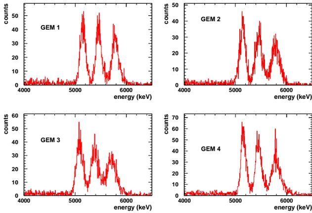
Fig. 2. Energy resolution as obtained with the gas electron multipliers and a triple- $\alpha$  source. For these measurements, the source was mounted just outside the active volume of the TPC. The  $\alpha$  particles were emitted parallel to the detection plane and collimated with a collimator of length 3 mm and an opening of 1 mm. The measurement was performed at 500 mbar of P10 (90% Ar - 10% CH<sub>4</sub>) with a high voltage of 320 V across the GEMs.
