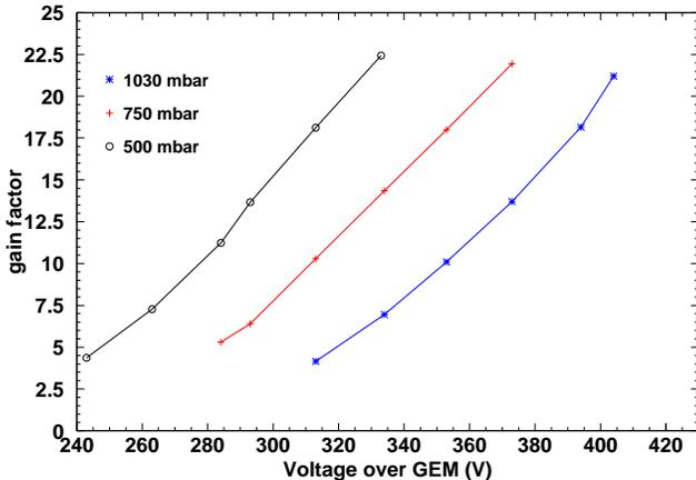
Fig. 3. The figure shows the gains measured for different pressure regimes. The gains were measured with two GEMs and are defined as the ratio between the signals measured on the second GEM and the first GEM. The distance between the GEMs was 10 mm.
