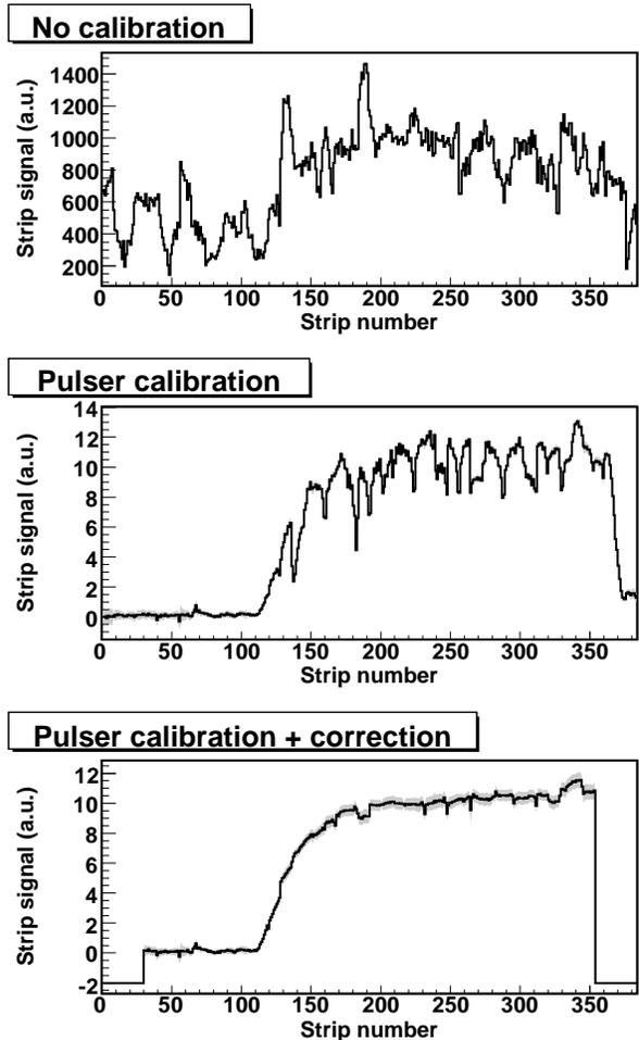
Fig. 6. The signal registered by each strip perpendicular to the beam is shown from an implantation event. The upper spectrum shows the ASIC response without calibration, the center spectrum with the pulser calibration described in the text, and the lower figure with the additional correction by means of the traversing beams. The smoothing procedure is not yet applied for these spectra (see text for details). The shaded area indicates the error bars.
