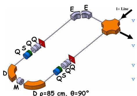
The quadrupole doublet matching section produces a ribbon-shaped beam, so y-angles are small, minimizing b aberrations
